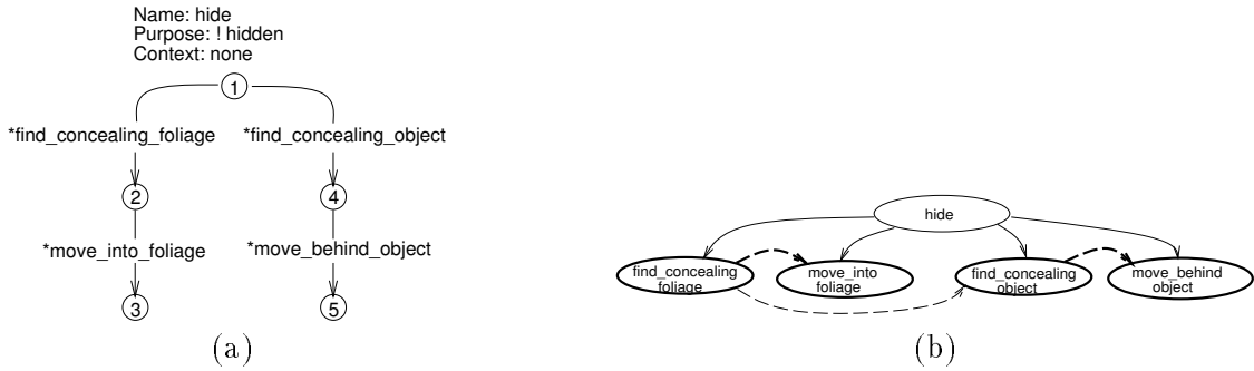
Figure 3: (a) Single plan with OR branch. (b) Corresponding belief network.
